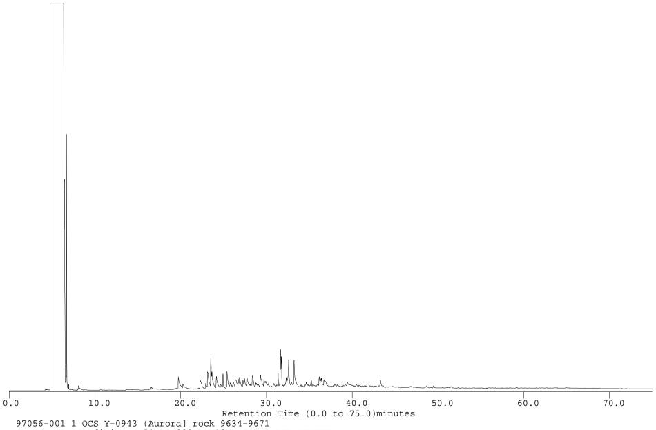
97056-001 1 OCS Y-0943 (Aurora] rock 9634-9671 Instrument Conditions: 50 TO 320 AT 10 DEGREES PER MINUTE Method: arom`mth, Low Scale=2.213 mV High Scale=999.999 mV 97056A01.raw, Analyzed: 11/17/97 by U.S.G.S. Box 25046 MS 977 Denver, CO 80225
